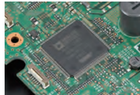
For band scope ADSP-21363 clock @333 MHz
