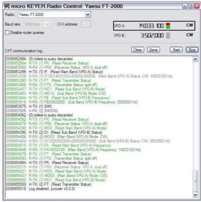
**<u>TIP:</u>** Disable the Autobaud function in any Icom Radio used with Router. Configure the radio, Router, and your application software to operate at 9600 or 19200 baud.
